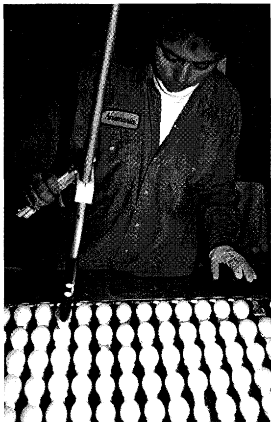
Left: An example of high tech equipment at work protecting the food supply. A Fassio Egg Farms employee uses an electronic "wand" to mark cracked or damaged eggs that will later be removed by computer.
